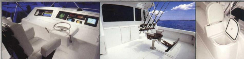
**Main photo: Top speed was 47.7 mph during our sea trials. Inset photos, left to right: The Viking has electronics lockers at the helm with clear, watertight hatches. The Bluewater fighting chair is optional. And check out this seat on the bridge; the back flips around so you can face forward or aft.**
