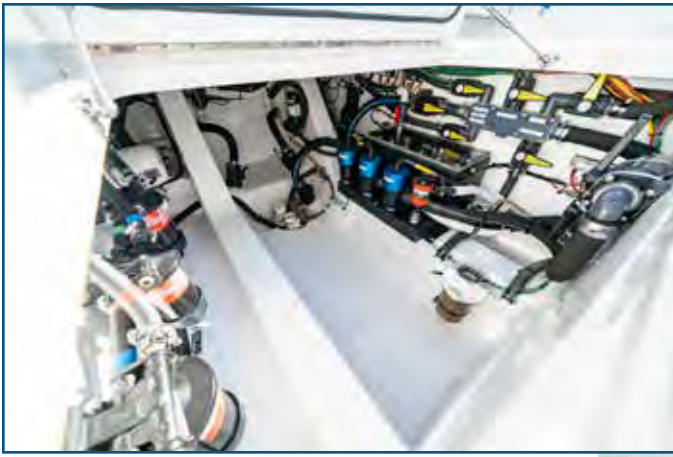
Clockwise from top left: Trust Fun's immaculate Snow White lazarette with sea chest system; the machinery room with 12kW genset, Koden broadband searchlight sonar, battery boxes and other mechanical, electrical and plumbing components; and the Seakeeper 6 mounted in its engineered location forward of the lazarette.
