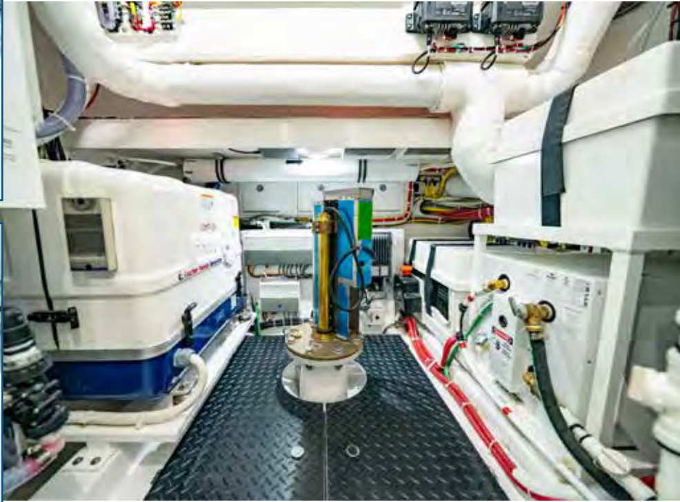
Clockwise from top left: Trust Fun's immaculate Snow White lazarette with sea chest system; the machinery room with 12kW genset, Koden broadband searchlight sonar, battery boxes and other mechanical, electrical and plumbing components; and the Seakeeper 6 mounted in its engineered location forward of the lazarette.
